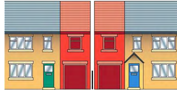
Figure 2: Side extensions to detached and semi-detached houses with no gap can cause the appearance of terraced housing which does not match the street scene.
