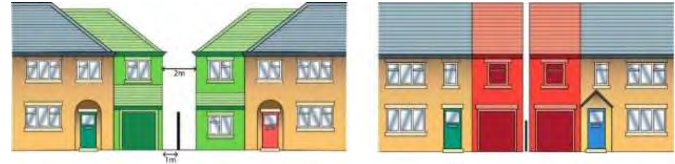
Figure 23: Left image shows two detached properties which include a 1m gap between the boundaries and are set back by 500mm from the building line to provide a lowered ridgeline. The right image shows a side extension to detached dwellings providing no gap between the buildings causing a terracing effect.
