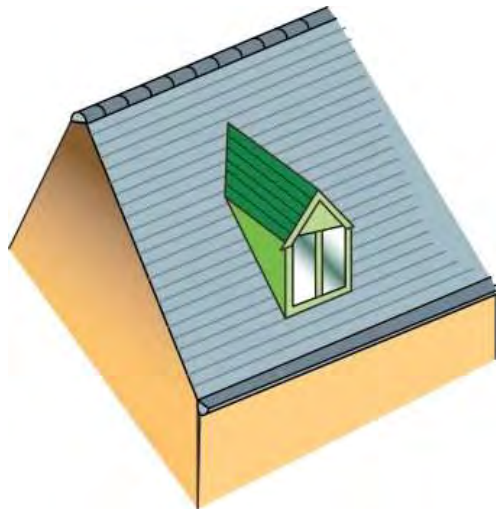
Figure 27: Example of a traditional vertical dormer which complements the existing pitched roof.
