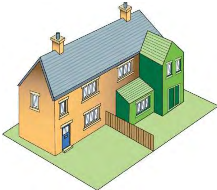
Figure 18: Acceptable part two storey part one storey rear extension which does not affect the neighbouring property.
